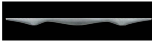
Figure 2.18: Concrete beam made with fabric formwork
