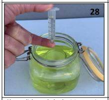
Close lid and lock Mason jar. Chlorine Dioxide gas off and infuse into distilled water.
